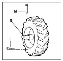
Fig. 2-3: Wheel in FREEWHEELING position (wheel drive pin through wheel shaft only).
